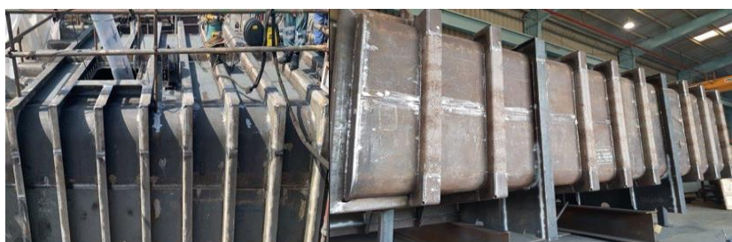
Figure (1) Typical arrangement and construction details of Well Stimulation HCl Acid Tanks located under deck [Courtesy of OML (Overseas Marine Logistics L.L.C.)]
